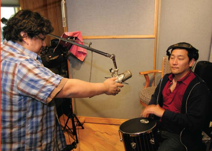
A multitalented engineer and mixer, Robert Carranza is widely known and respected for his work with such artists as Los Lobos, Ozomatli, Jack Johnson, Beck, Eels, Molotov and Supergrass. To record Jiro Yamaguchi's drum, Carranza adjusts a Neumann U47, which goes through a Chandler Limited TG Channel MkII preamp.
